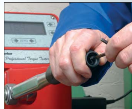
'P' Type wrenches have no scale. They must be set against a torque testing device such as Norbar's Professional Torque Tester (see page 68).
