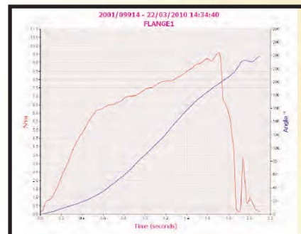
Torque and Angle vs Time graph produced using T-Box MS software
